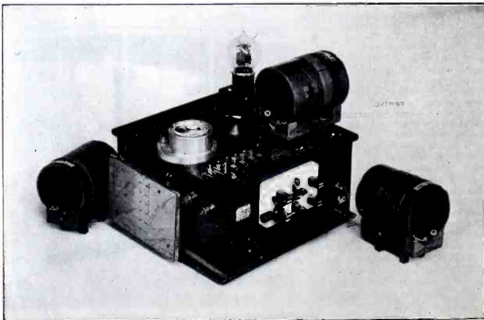
The Arrangement Here Shown Is a Simple Short-Wave Generating Set Using a Small Vacuum Tube.
